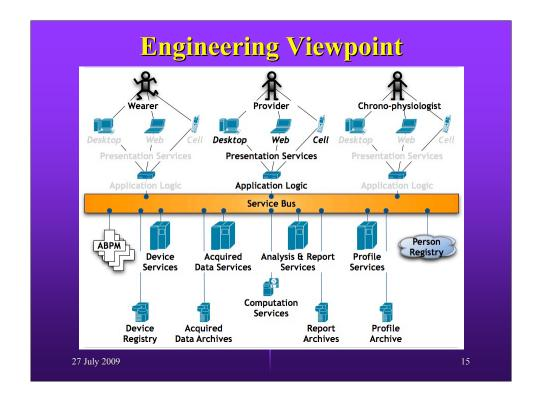
The whole system is hung together off a "Service Bus"
